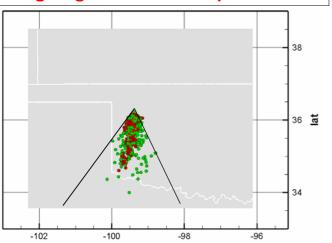
Lagrangian particle dispersion using the average wind field with & without accommodations for wind direction uncertainty. The "without" dispersion aligns with the low-uncertainty core, while the "with" fills in the high-uncertainty fringes (see Plume Unc. figure).
